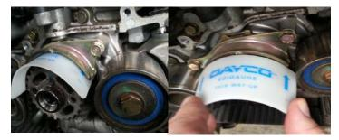
EZIGAUGE does not fit between the timing belt and the guide plate (where fitted) then loosen the guide plate retaining bolts and adjust the guide so the EZIGAUGE fits. **Only remove the EZIGAUGE after both bolts on the guide plate have been tightened.**
