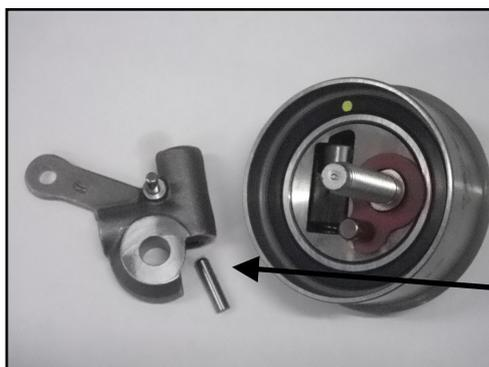
Rod actuator is separated from hydraulic sub-assembly
