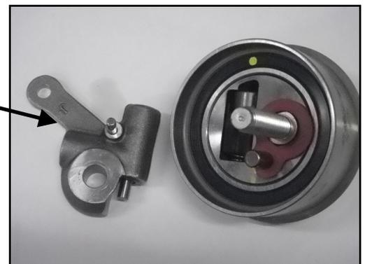
Hydraulic sub-assembly is separated from main body
