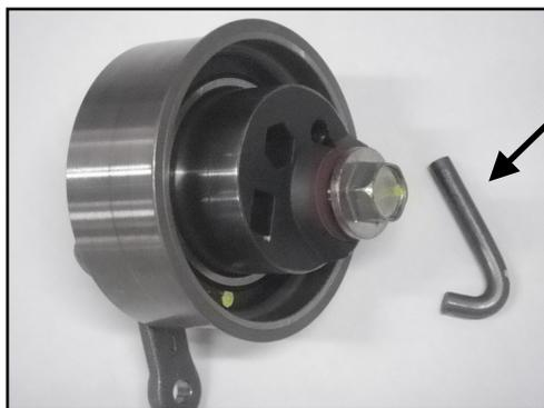
Retainer pin is loose or separated from main assembly
